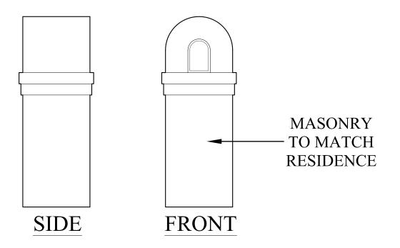
Mailbox shall be approximately 16 brick courses high with the mail box being approximately 38" to 42" above street level. All mortar joints shall be 3/8" All course batts are cut so no holes are exposed
